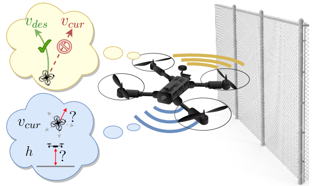
Figure 1: A downward facing radar performs altimetry and ego-velocity estimation (bottom) and a forward facing radar performs collision avoidance (top), removing the need for other exteroceptive sensors such as cameras or lidar.
